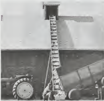
Flight grain elevator moving ear corn into a crib in a barn
